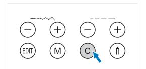
Press this button when the incorrect character is selected. Each press of this button erases one character, or press this button to remove an added pattern when sewing combinations of characters or decorative stitches.
