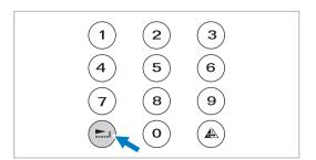
The LED light will be set at direct mode "  $\S$  " when start the machine. By pressing the button, LED light will move step by step to select the stitch mode, as shown.
